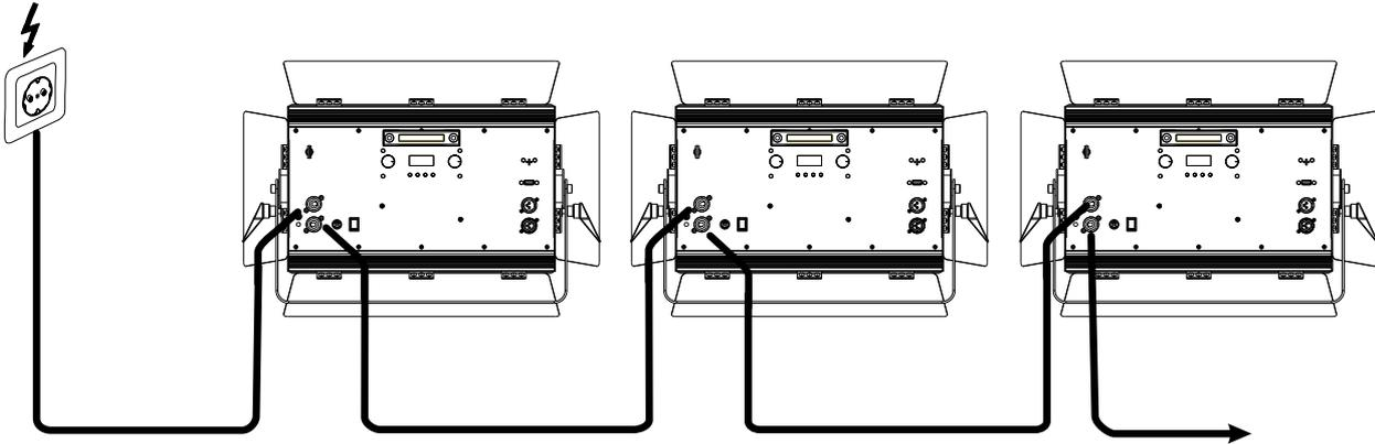
The device uses an auto-range power supply that accepts input voltages between 100 und 240 volts.
